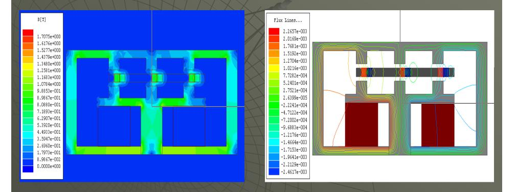
Shading in above figure represents magnetic field, lines represent magnetic flux
